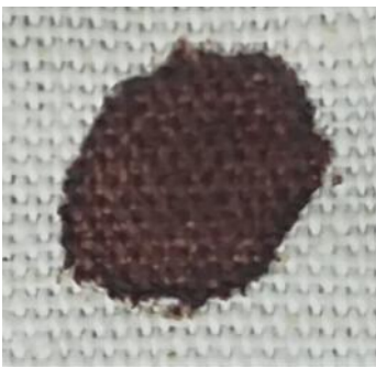
Fig. 3. High bilirubin blood stain just after lamp irradiation with a UV dose below threshold for both linen coloration and latent coloration. The blood stain appears undamaged.
